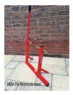
The ABBA Stand uses the swing arm pivot to attach it to your bike. It locks to both sides of your bike, ensuring rock solid security when your bike is fitted to the stand.
